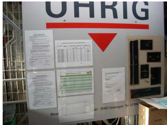
Figure 5.1 Work station with table of tolerance requirement and examples of gaskets defects
