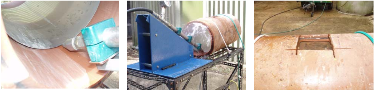
Figure 1 Testing of tapered end of repair
