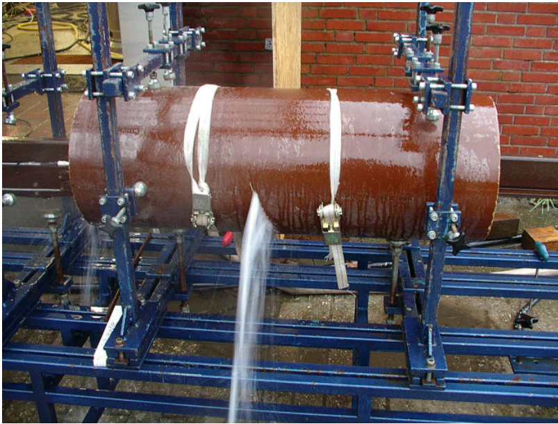
Fig. 5: test specimen with placed gasket installed in test-stand
